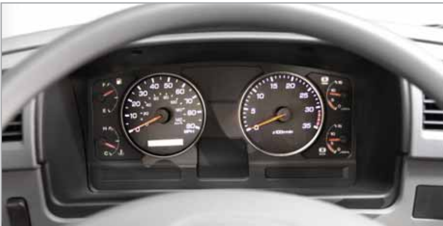
Revised instrument panel layout gives driver quick view of engine status
